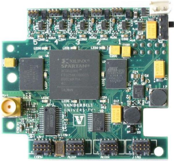
**Figure 5: FPGA-based sensor board**
